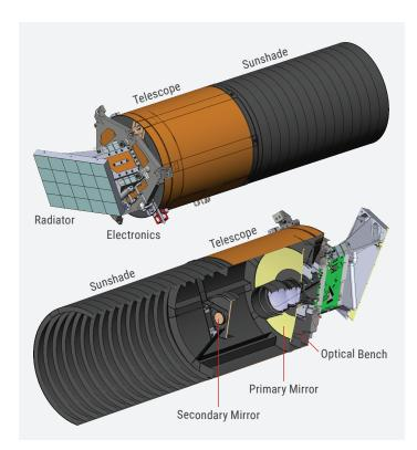
Labeled drawing of the ShadowCam instrument (top) and cross-section (bottom) showing the internal optics and mirrors.
